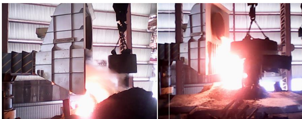
Figure 6.14: Working of side-based Suction Hood
